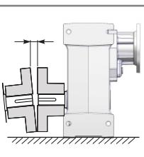
Check shaft and coupling alignment. Check proper coupling gap before to lock all foundation bolts that should be routinely checked.
