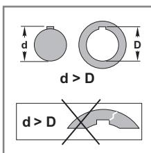
When mounting items to the reducer shaft, appropriate anti-seize and oxidizer compounds should be used, and key dimensions are concerned.
