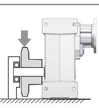
For very heavy radial load, additional output shaft support may be required to prevent premature bearing failure or shaft breakage from bending fatigue.
