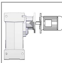
When mounting a motor to reducers, the fastening bolts should not be tightened until both the reducer flange and motor face are in contact. When mounting is complete check by manually rotating the fan to be sure the assembly turns freely.
