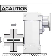
The system of connected rotating parts must be free from critical speed, torsional or other type vibration, no matter how induced. The responsibility for this system analysis lies with the purchaser of the speed reducer.
