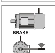
Reducers are not to be considered fail safe or self-locking devices. If these features are required, a properly sized, independent holding device should be used. Reducers should not be used as a brake. Any brakes that are used in conjunction with a reducer must be sized or positioned in such a way so as to not subject the reducer to loads beyond the catalog rating.
