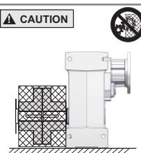
For safety, Buyer or User should provide protective guards over all shaft extensions and any moving apparatus mounted thereon. The User is responsible for checking all applicable safety codes in his area and providing suitable guards. Failure to do so may result in bodily injury and/or damage to equipment.
