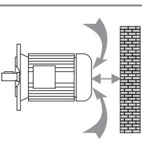
Make sure there is sufficient space between any obstructions and the motor's air intake area to provide adequate cooling for the motor.
