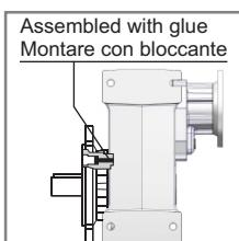
In applications where multiple starts, stops or reverses occurs, it is recommended to block the fastening bolts of the output flange and feet.
