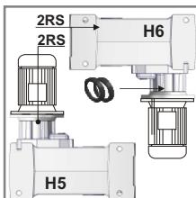
Do not change mounting positions without contacting our factory. Altering the mounting position may require special lubrication provisions which must be installed from the factory. When reducers are mounted in positions H5 or H6 and used in continuous duty applications, replace the upper bearing with a self lubricated style bearing, and we suggest double input seal for H6.
