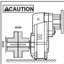
The system of connected rotating parts must be free from critical speed, torsional or other type vibration, no matter how induced. The responsibility for this system analysis lies with the purchaser of the speed reducer.
