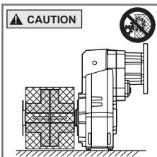
For safety, Buyer or User should provide protective guards over all shaft extensions and any moving apparatus mounted thereon. The User is responsible for checking all applicable safety codes in his area and providing suitable guards. Failure to do so may result in bodily injury and/or damage to equipment.
