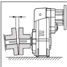
Check shaft and coupling alignment. Check proper coupling gap before to lock all foundation bolts that should be routinely checked.
