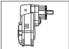
**2** A gear box version R (or B) is to be found from the selection tables, considering the required power  $P_{1r}$  (or torque  $M_{2r}$  required) and output speed  $n_2$  referred to  $1400 \text{ min}^{-1}$  (or to gearbox ratio).
