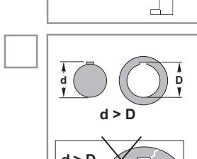
When mounting items to the reducer shaft, appropriate anti-seize and oxidizer compounds should be used, and keys dimensions are connected.
