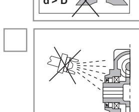
If the reducer is to be painted, protect machined surfaces and oil seals from over-spray.
