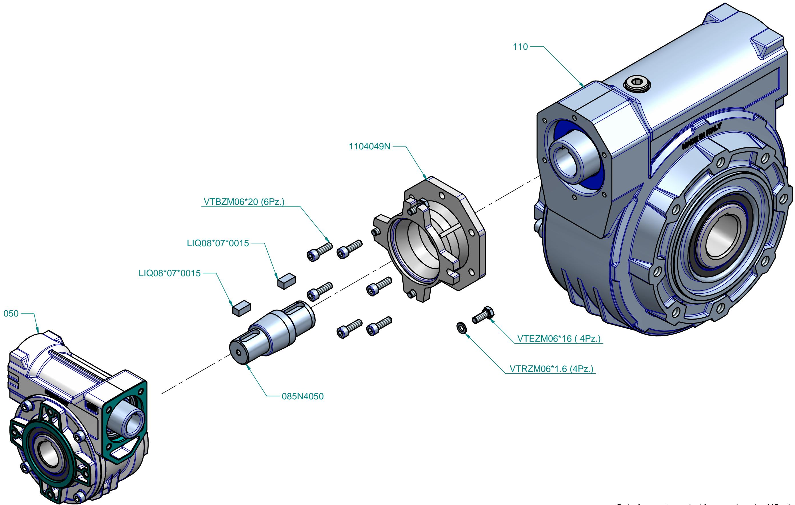
Order from parts required from gearbox size **115** ratio \_\_\_\_\_
