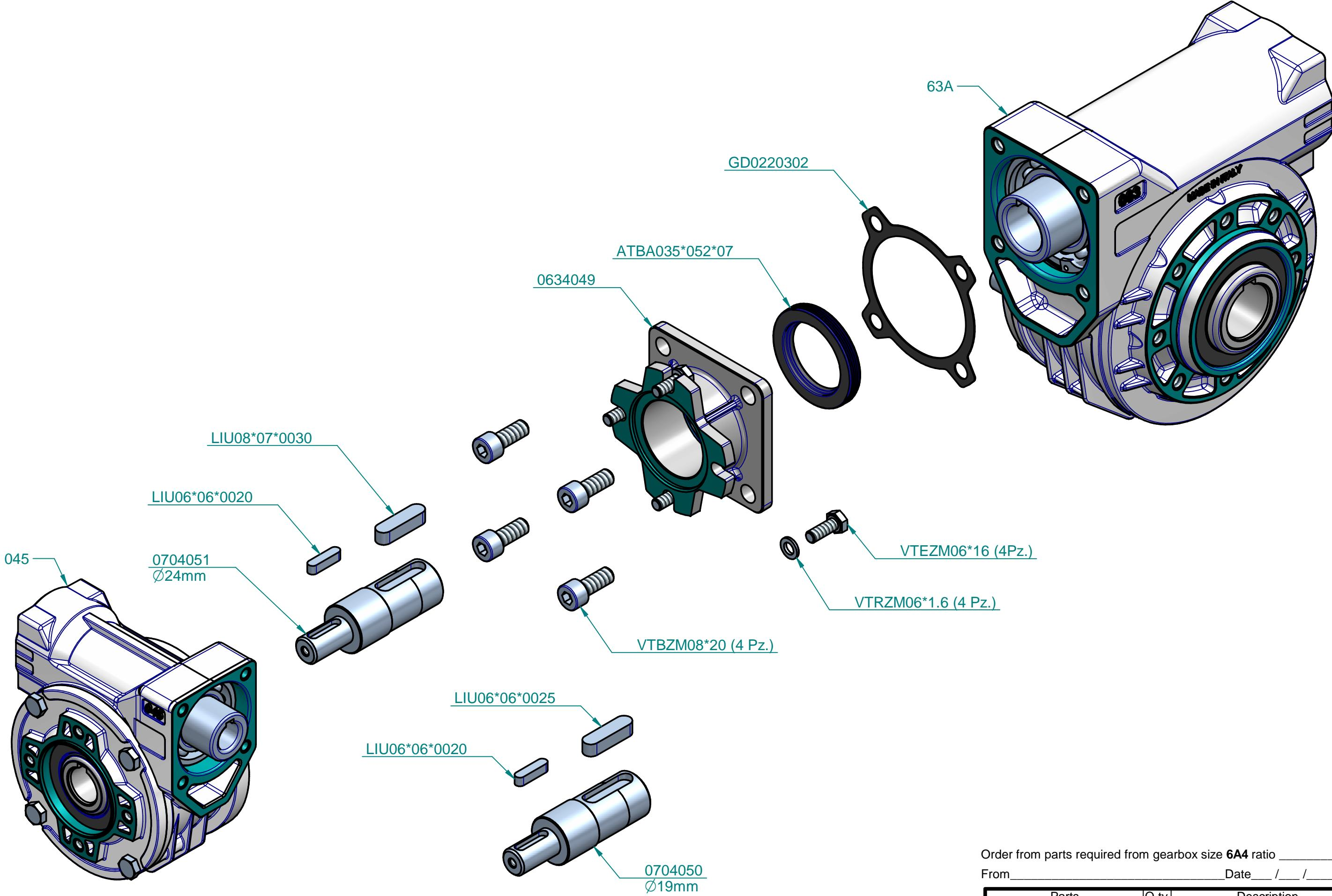
Order from parts required from gearbox size **6A4** ratio \_\_\_\_\_
