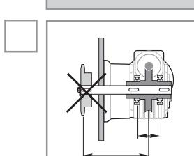
Make sure that mounting of pulleys or pinions does not create overhung loads exceeding the capacity of the reducer.
