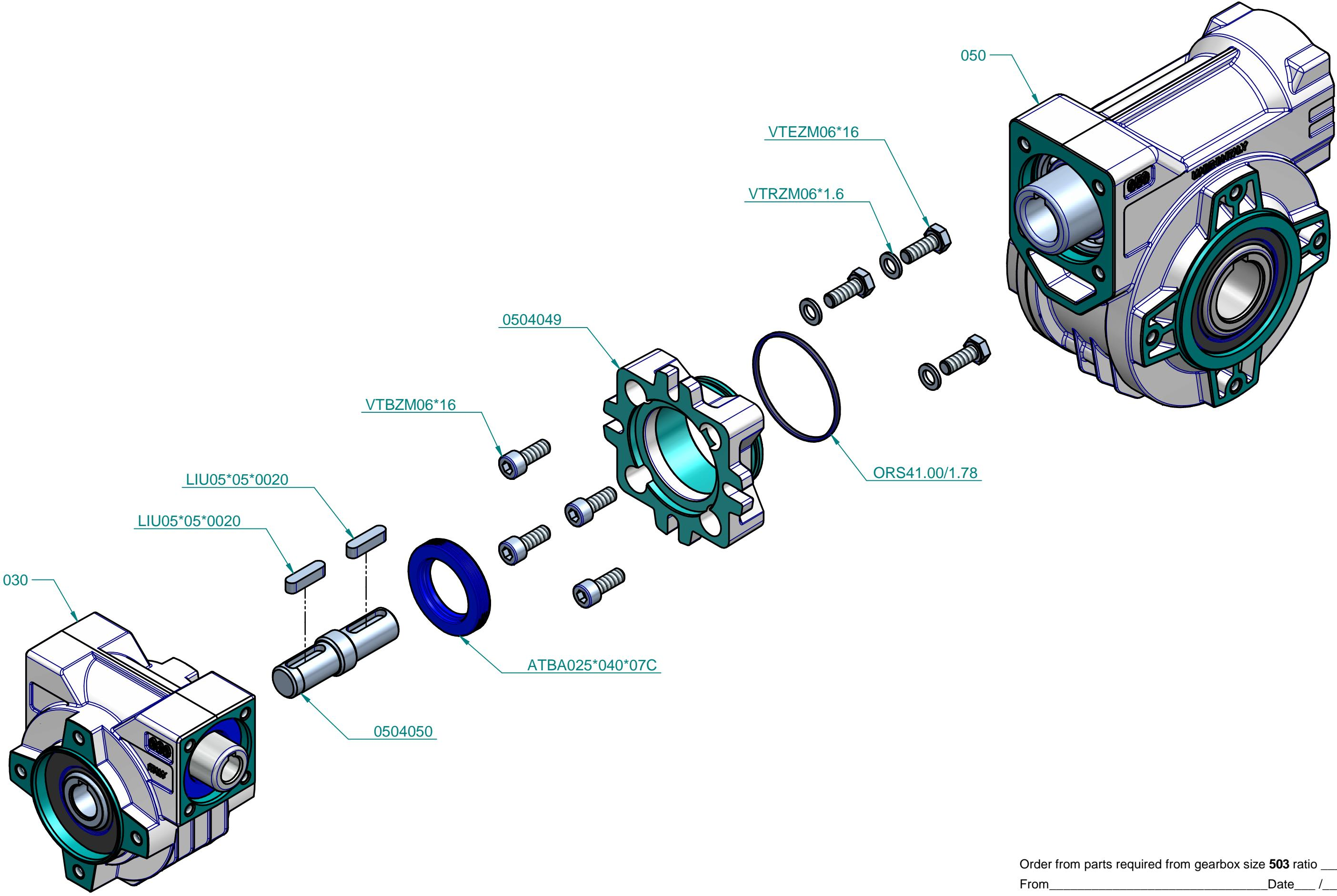
Order from parts required from gearbox size **503** ratio \_\_\_\_\_
