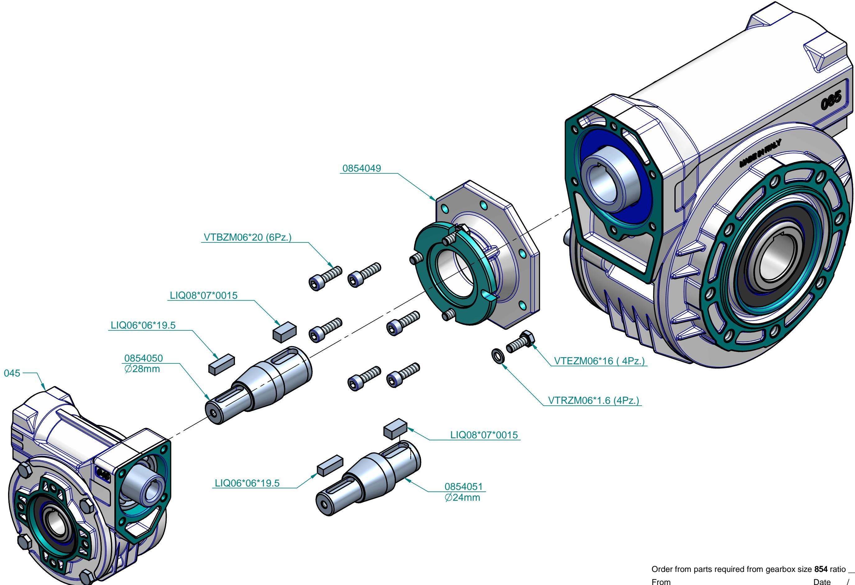
Order from parts required from gearbox size **854** ratio \_\_\_\_\_
