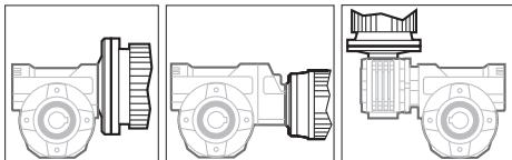
**4** Motorized gear boxes (version M) can be easily selected throughout the appropriate selection tables.
