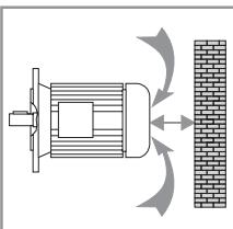
Make sure there is sufficient space between any obstructions and the motor's air intake area to provide adequate cooling for the motor.
