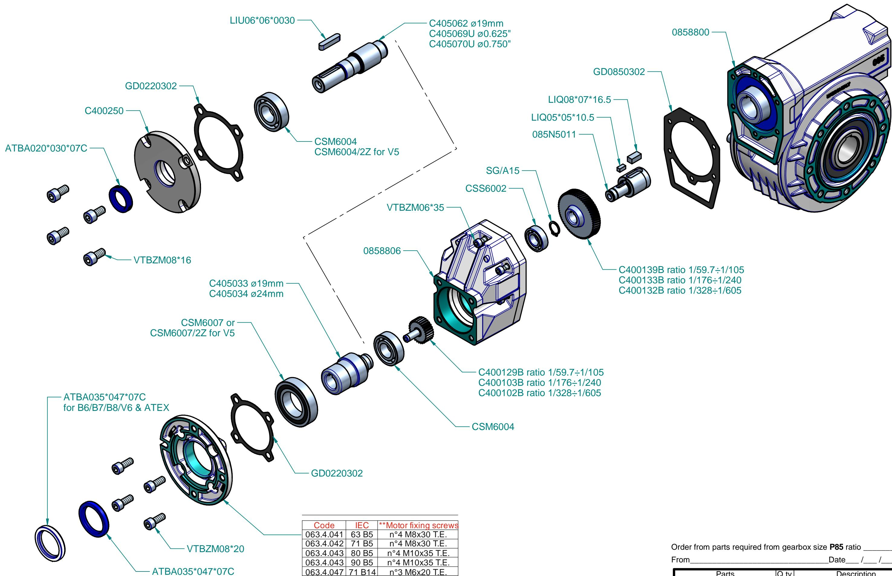
Order from parts required from gearbox size **P85** ratio \_\_\_\_\_
