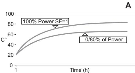
Worm gearboxes, because of their inside design, transform part of their installed power into heat which is subsequently disposed of throughout the housing and may result into values, measured onto the gear case in the area of the worm shaft, in the range of 80 - 100 °C without this affecting the operation of the gear unit adversely.
