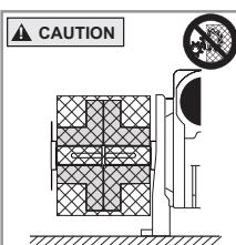
For safety, Buyer or User should provide protective guards over all shaft extensions and any moving apparatus mounted thereon. The User is responsible for checking all applicable safety codes in his area and providing suitable guards. Failure to do so may result in bodily injury and/or damage to equipment.
