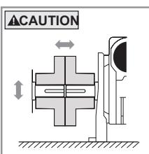
The system of connected rotating parts must be free from critical speed, torsional or other type vibration, no matter how induced. The responsibility for this system analysis lies with the purchaser of the speed reducer.
