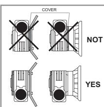
In case of high loads do not fix the gearbox on its side cover (FB). It is recommended instead to use the opposite side as, in such a way, the gearbox fixing is carried out directly on the housing in a safer way.
