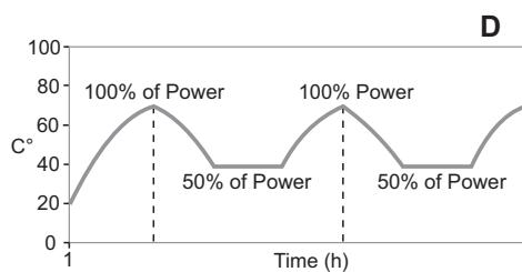
Geared motor selections with 2800 min-1 input speed are tolerated for intermittent duty applications only, because of the high temperature increase resulting from the input rotation speed.
