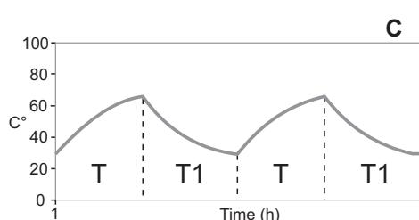
Should the gearbox have several starts and stops cycles, the final temperature depends on starts and stops times (very similar to electric motors with operation S3 and S6 see graphs C and D). Service factor values indicated in this catalogue refer to an intermittent duty.
