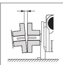
Check shaft and coupling alignment. Check proper coupling gap before to lock all foundation bolts that should be routinely checked.
