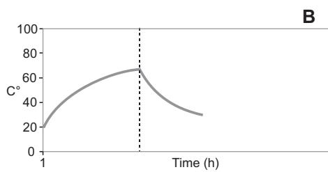
In this case the temperature increase curve is similar to the one for continuous duty. In fact the peak is reached in approximately 20/30 min utes using 100% of the power.
